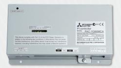
The PAC-YG60MCA Pulse Input (PI) Controller makes it possible to perform energy saving and energy allocation initiatives. A maximum of four (4) measurement meters (WHM, gas meter, water meter, and calorie meter) can be connected to the PI Controller and trended within the Centralized Controller. (Note: 24VDC power needs to be provided on-site.)
